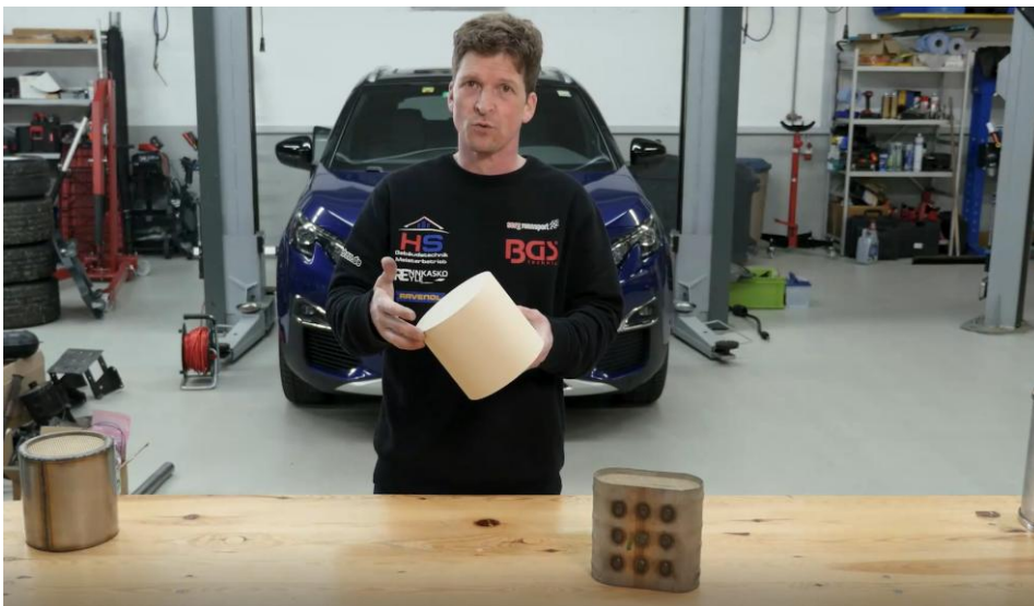
Figure 4 Screenshot VERT's Video - new technology developed with very fine porosity to clean petrol exhaust gases. (03:48)
