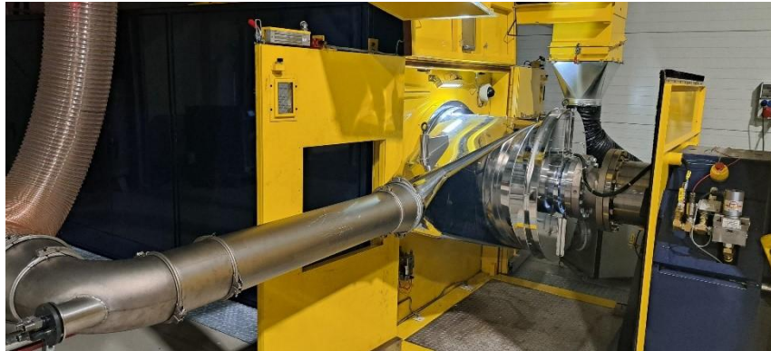
Figure 1: Brake enclosure for emission measurements on the CV dynamometer
