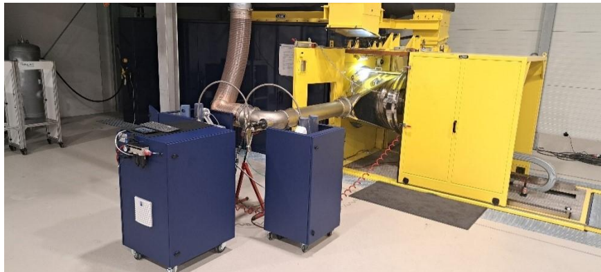
Figure 3: Experimental setup for commercial vehicle brake emission measurements consisting of the dynamometer, brake enclosure, sample duct, sample elbow, devices for measurement of particle number (total and solid), particle mass (PM 2.5 and PM 10 ).
