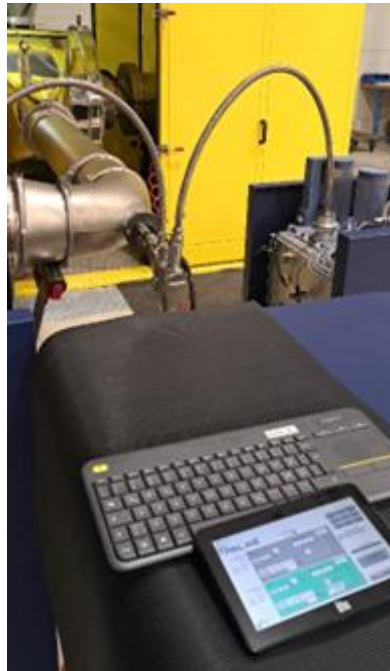
Figure 5: Emission Enclosure with sample elbow, PM cyclones, sampling tubes and control display for the M4222-PN
