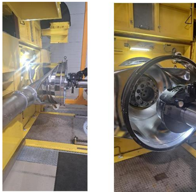
Figure 2: Detailed view on the emission enclosure with sample duct (left) and brake assembly (right)
