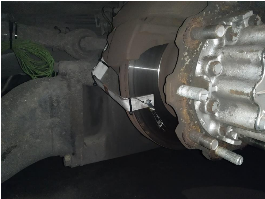
Figure 6: Thermocouple installed at the brake
