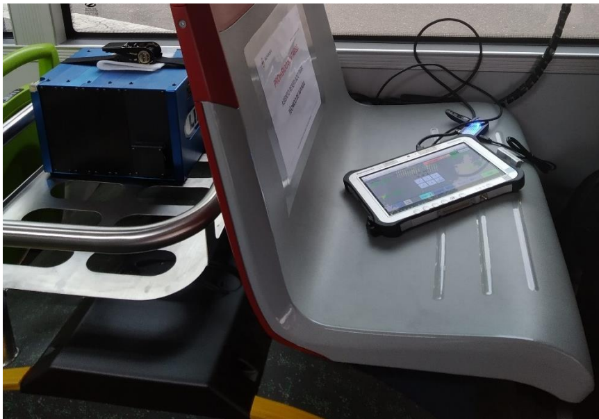
Figure 4: LINK VMAX fixed in longitudinal direction to the bus (left) and Control Screen (right)
