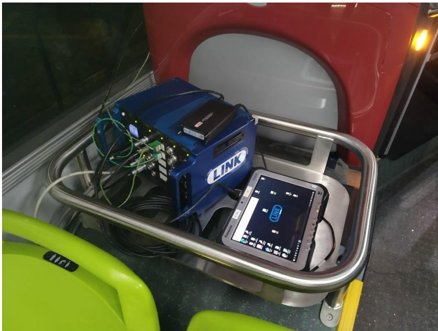
Figure 2: LINK VMAX Data Acquisition System
